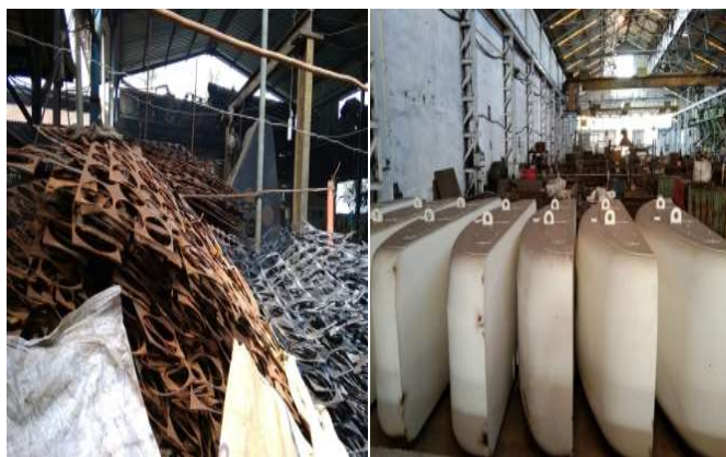
Fig. 7. Iron scrap from metal cutting (Left) and after-utilization as counterweight (Right)
